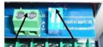
Terminal strip J22 Toggle switches
